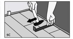
There must also be a 1/4" to 3/8" (6.35mm to 10 mm) expansion joint between the last row and the wall. Keep this in mind when sawing the last row of panels.
